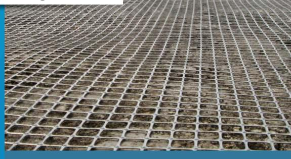
Fortech EG Bi-Axial Geogrid, are high modulus polypropylene geogrids, produced by an extrusion process offering tensile resistance both in the longitudinal and in the transverse direction.
